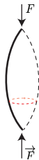
(c) Spontaneously broken symmetry: the rod bends in an arbitrary direction and loses rotational invariance
