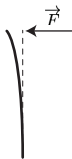
(b) Explicitly broken symmetry: the rod bends due to an external force and loses rotational invariance
