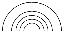
TE_{01} mode. E -lines in AB section spaced to give equal intensity increments.
