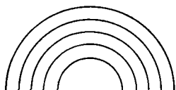
TM_{01} mode. B -lines in AB section spaced to give equal induction increments.
