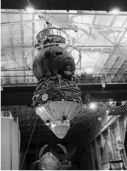
**Fig. 11.6** *Foton 12* spacecraft carried to the Soyuz launcher, in the MIK integration facility at Plesetsk Cosmodrome (Russia) in September 1999 (photo credit: ESA).
