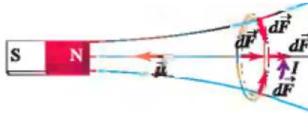
(b) Net force on same coil is toward south pole of magnet.
