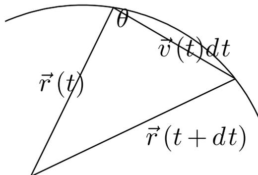
$$dA = \frac{1}{2}r(t)v(t)\text{sen } \theta dt. \frac{dA}{dt} = \frac{1}{2}|\vec{r}(t) \times \vec{v}(t)| = \text{constante}$$
