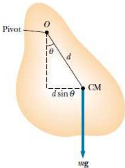
$$\begin{aligned}\tau &= -mgd \sin\theta = I_o \ddot{\theta} & I_o &= I_{CM} + Md^2 \\ I_o \ddot{\theta} &= -mgd \theta \quad \theta \ll 1 \\ \omega &= \sqrt{\frac{mgd}{I_o}}\end{aligned}$$
