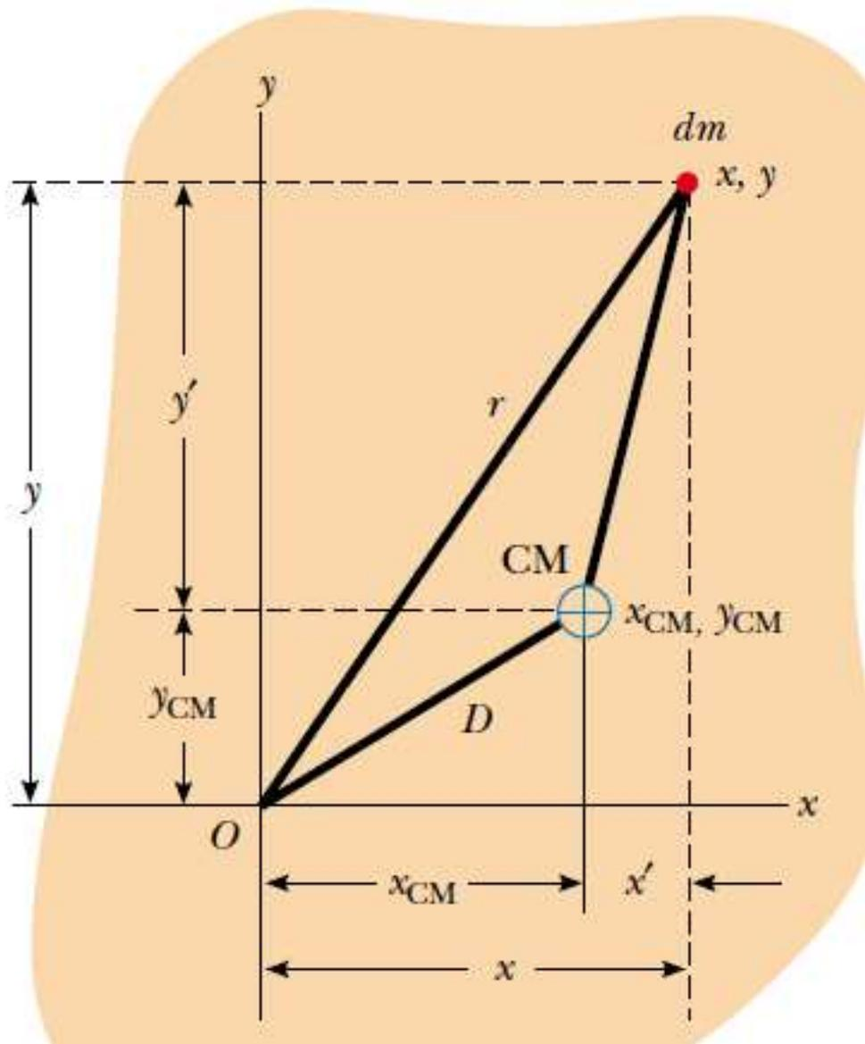
$$I = \int dm(x^2 + y^2) \quad x = x_{\text{CM}} + x' \quad y = y_{\text{CM}} + y'$$
