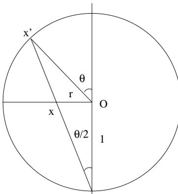
FIGURE 1. Relation between stereographic projection and geodesic coordinates
